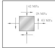
For the given state of stress, determine (a) the orientation of the planes of maximum in-plane shearing stress, (b) the corresponding normal stress.
