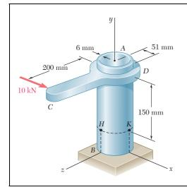
The steel pipe AB has a 102-mm outer diameter and a 6-mm wall thickness. Knowing that arm CD is rigidly attached to the pipe, determine the principal stresses and the maximum shearing stress at point K.
