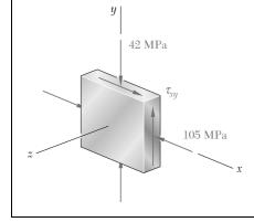
For the state of stress shown, determine the value of  $\tau_{xy}$  for which the maximum shearing stress is (a) 63 MPa, (b) 84 MPa.
