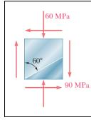
For the given state of stress, determine the normal and shearing stresses exerted on the oblique face of the shaded triangular element shown. Use a method of analysis based on the equilibrium of that element, as was done in the derivations of Sec. 7.1A.
