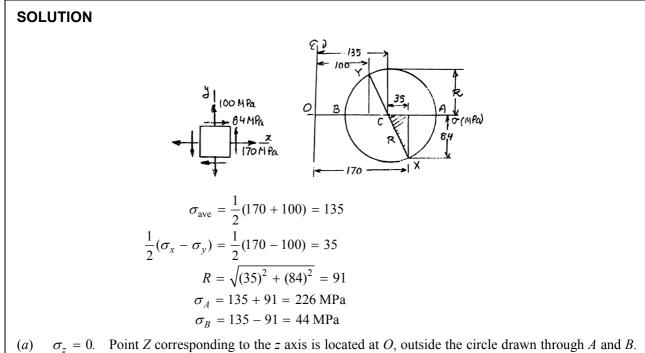
(a)  $\sigma_z = 0$ . Point Z corresponding to the z axis is located at O, outside the circle drawn through A and B. The largest of the 3 Mohr's circles is the circle through O and A. We have
