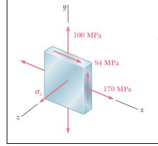
For the state of stress shown, determine the maximum shearing stress when (a)  $\sigma_z = 0$ , (b)  $\sigma_z = +60$  MPa, (c)  $\sigma_z = -60$  MPa.
