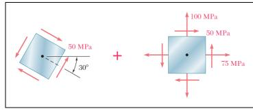
Determine the principal planes and the principal stresses for the state of plane stress resulting from the superposition of the two states of stress shown.
