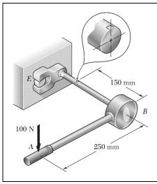
A mechanic uses a crowfoot wrench to loosen a bolt at E. Knowing that the mechanic applies a vertical 100 N force at A, determine the principal stresses and the maximum shearing stress at point H located as shown on top of the 18 mm diameter shaft.
