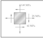
For the given state of stress, determine (*a*) the principal planes, (*b*) the principal stresses.
