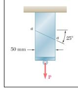
Two members of uniform cross section  $50 \times 80$  mm are glued together along plane *a-a* that forms an angle of 25° with the horizontal. Knowing that the allowable stresses for the glued joint are  $\sigma = 800$  kPa and  $\tau = 600$  kPa, determine the largest centric load **P** that can be applied.
